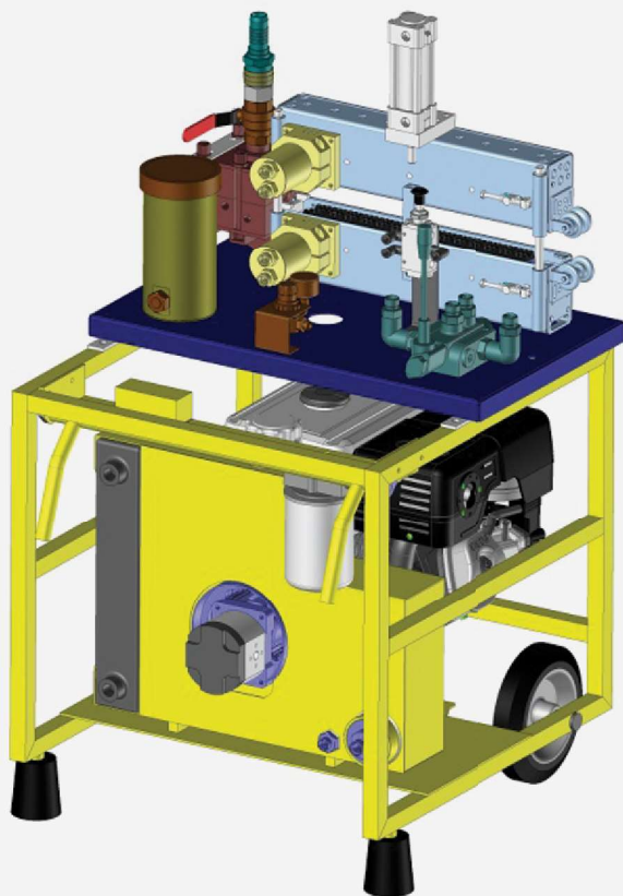
Hydraulic Fiber Blowing Machine
